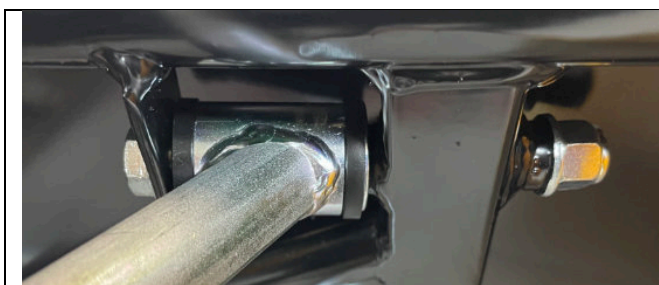
Rear showing white bushings in lower wishbones
